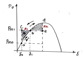
A sudden step increase in input power represented by the thorizondal line,  $Pm_1$ . Since  $Pm_1 > Pe$ , the accelerating power Pe,  $Pa = Pm_1 - Pe$  on the noton is positive and the power angle  $\delta$  increases and the noton speed increases. The encess energy stored in the noton during the initral acceleration is,
