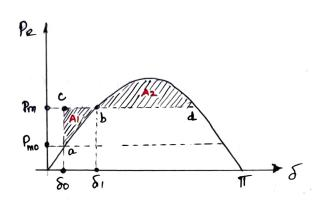
If area A2 / Area A1, the accelerating momentum can never be over come. The limit of stability occurs when Smax is at the entersection of Pm and the power angle arrive for 90 / 8 / 180.
