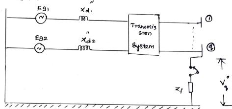
Let us assume 3 p fault occurs at bus q through a foult impedence  $X_f$ .
