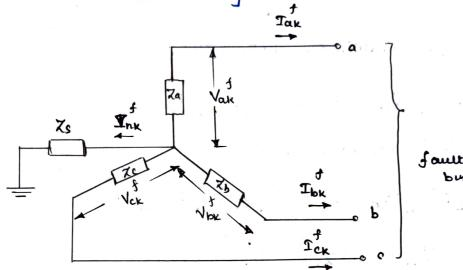
For a solid L-1 fault with simultaneous ground contact,
