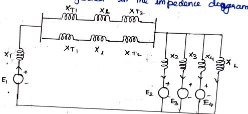
Bus Admittance Matrix or Y-bus matrix finds application in load flow and optimal load flow analysis as well as stability analysis. Z-bus matrix or Bus impedence matrix finds application in short circuit analysis.
