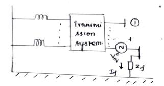
The current entening every bus is zero except at the faulted bus.
