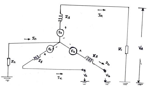
suppose a line to ground fault on phase a connected to ground through impedence of Assume the generator is initially on no load, the conductors at the fault bus k are empressed as
