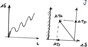
With continuously acting voltage regulators, the small disturbance stability problem is one of ensuring suffraent damping of oscillations. Instability is normally through oscillations of increasing amplitude.
