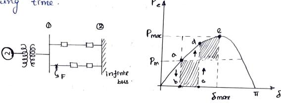
The angle of can be found that Area A1 = Area A2 the system is found to be stable. The system finally settles down to the steady operating point a Pn an oscillatory manner because of inherent damping. At point a, Pm = Pe.
