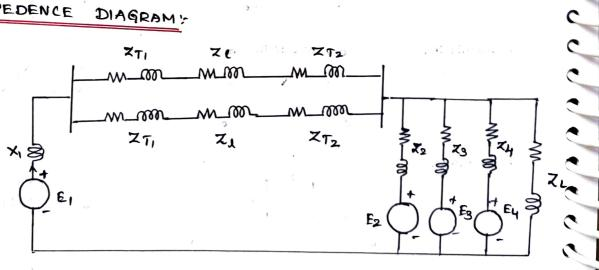
\* Single phase transformes equivalent execuit are shown as ideal transformer with transformer impedence indicated on approximate side.
