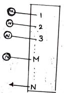
Consider N' bus system. Bus 1 to M are machine orc generator bus. Bus M+1 to N load buses.
