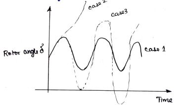
case (i): In the stable case, the notor angle Pricreases to a maximum, then decreases and oscillates with decreasing amplitude untill it reaches a steady state.
