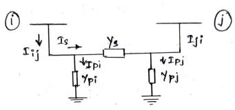
can be represented by the series admittance Ys and the two shunt admittances (half line charging admittance)
