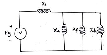
During initial part of the short curcuit, the damper and field windings have transformer secondary currents induced in Them whose primary is the aimatuse winding.
