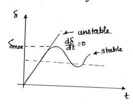
This is possible if the possitive (accelerating) area under Pa-8 curve is equal to the negative (decelerating) area under Pa-8 curve for a finite change in 8. Hence the Stabolity criterian called equal area criterian.
