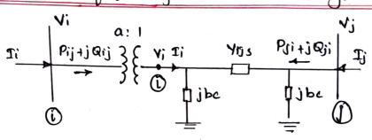
After finding complex bus voltages, the active and reactive flows in all the line/transformers are to be computed. A common II equivalent circuit for transmission line and transformer.
