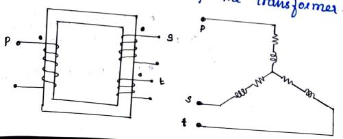
Let xps be the leakage impodence measured in primary with secondary short circuited and toritary open.
