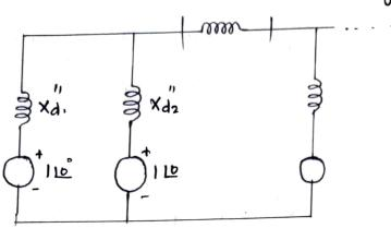
Assume one node as reference node and short circuiting all the voltage sources. Determine the Zbus using step by step bus building algorithm.
